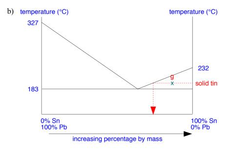
Draw a tie line through point g. It meets the 100% Sn axis, and so the mixture contains solid tin. Where it meets the other line, you can read off the composition of the molten liquid present.
